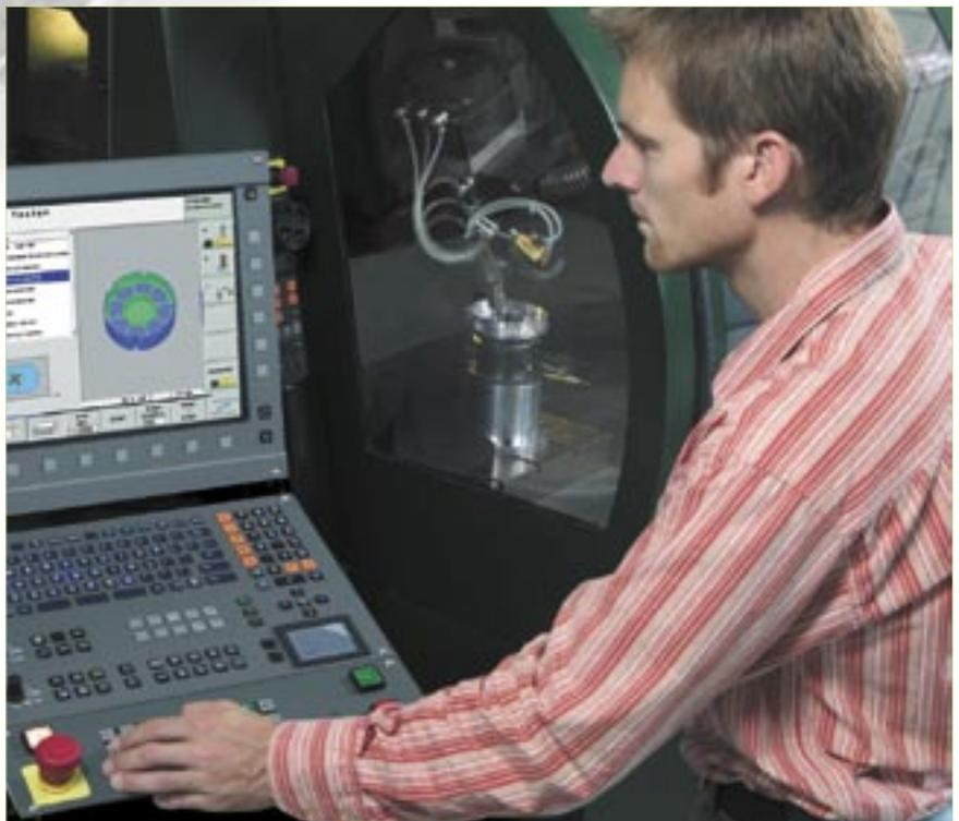
and texts. So that as little unnecessary information as possible appears on the screen during selection of the contours, you can hide via mouse click all excessive layers contained in the DXF file. This requires the keyboard with touchpad or an external pointing device. And here's the show-stopper when you select the contours later: The iTNC can select a contour train even if the designer has saved its parts on different layers.
