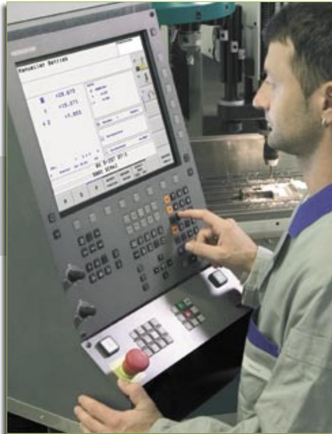
In order to keep set-up times as brief as possible, field-proven probing cycles are available in the Manual operating mode for you to quickly and accurately ascertain workpiece locations and orientations, as well as set reference points.
