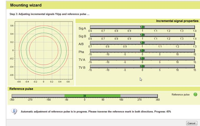
Move the encoder several times across the reference mark for an automatic adjustment of the incremental signal and the reference-mark signal. Note the Information and progress bar!
