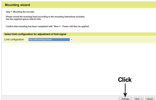
The adjustment of the reference-mark signal can be deselected if the encoder reference mark is not used.
