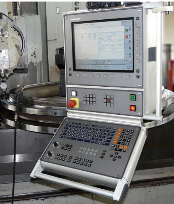
Machining of a generator shaft (eight metric tons) on a Zayer lateral milling machine controlled by an iTNC 530
