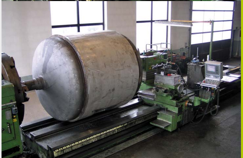
Flying lathe machining (above) Machining of a 2.1-m diameter mixing drum (below)
