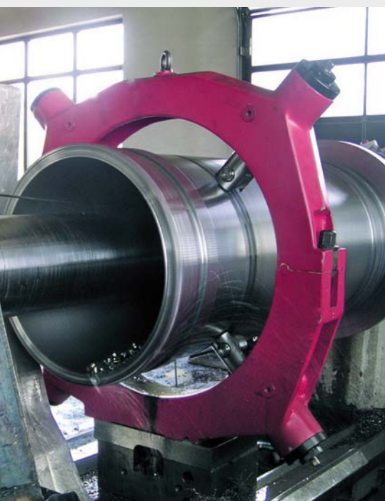
Internal machining of a tube for a centrifuge
