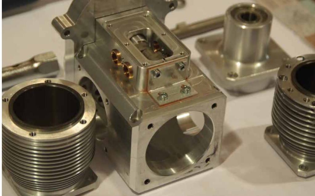
Components of a model-airplane engine manufactured on an iTNC 530
