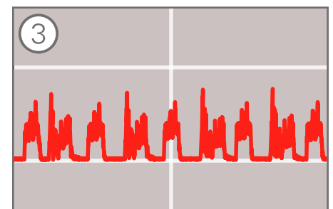
3 After 58 minutes with AFC: Spindle power at the time the AFC halts machining
